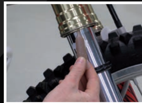
6. Apply grease between inner- and outertube
